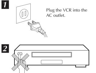
Don't press any buttons on the VCR or remote during auto setup.
